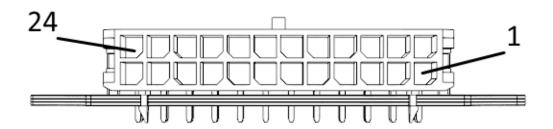
Converter has 12 contact pairs which are M-BUS interfaces. Converter provide connection up to 10 M-BUS devices. You can choose any 10 contact pairs. Wherein 1-2 contacts are M-BUS- (bot row), and 13-24 contacts are M-BUS+ (top row).
