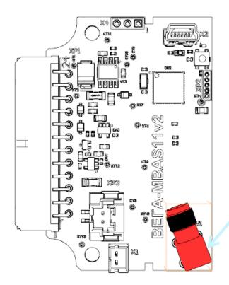
SMA connector for an external LoRaWAN antenna connection
